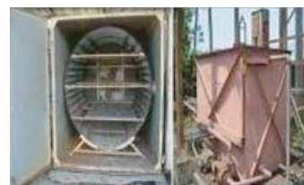
Moist hot air treatment plant
